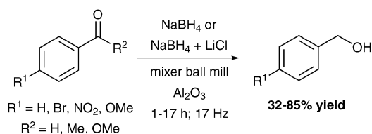
Scheme 13 Solid-state reduction of aryl carbonyl compounds to the corresponding benzylic alcohols. ¶
