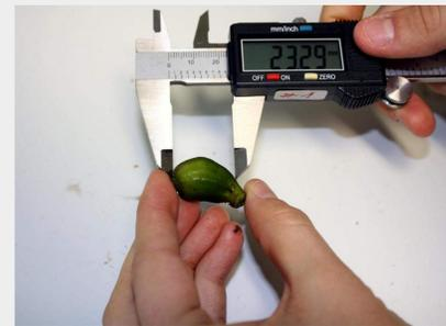
Figure 1: Measuring capsule dimensions
